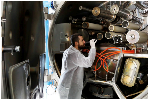
Roll-to-roll line for the production of flexible CIGS foil for customized PV, SunPlugged, Austria
